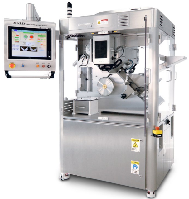
Ackley VIP Laser Drill with Brimrose AOTF-NIR
