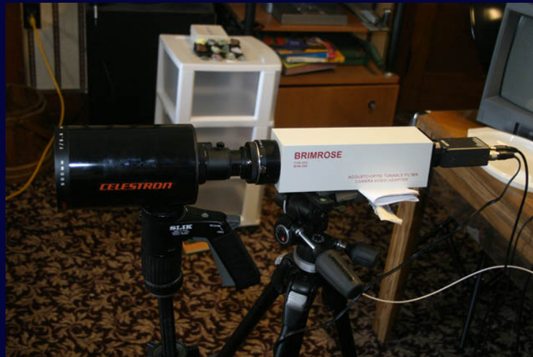
Imaging Spectrometer attached to a 9.25" F10 Schmidt Cassegrain Telescope:
