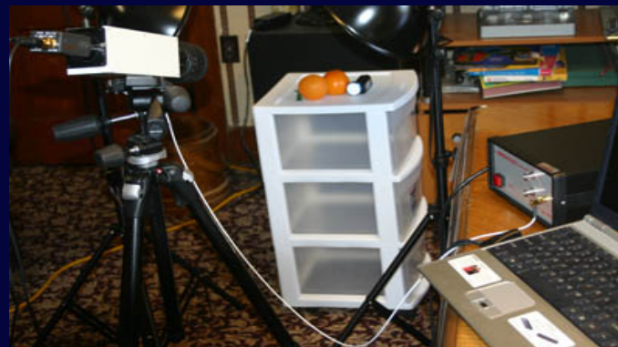
550 nm to 1000 nm Acousto-Optical Tunable Filter set up to take hyperspectral images of oranges
