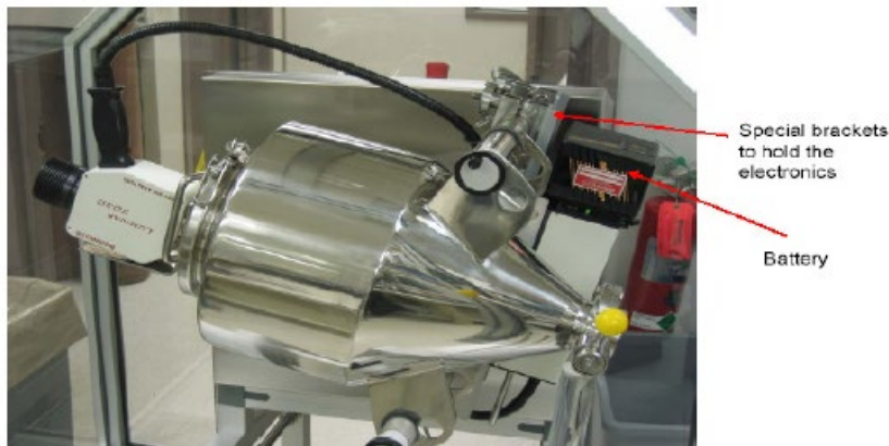
Image 1 - Handheld NIR system on a rotating drum in the laboratory
