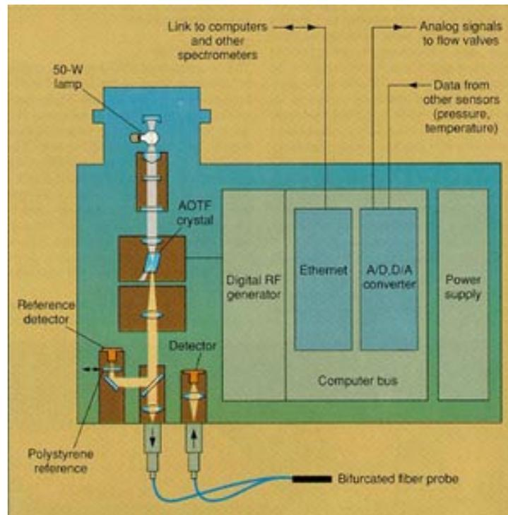
**Figure 2.** AOTF-based spectrometer integrates wavelength-tuning crystal in compact, all-solid-state device. Sampling with a bifurcated fiber probe makes the instrument adaptable to process environments.
