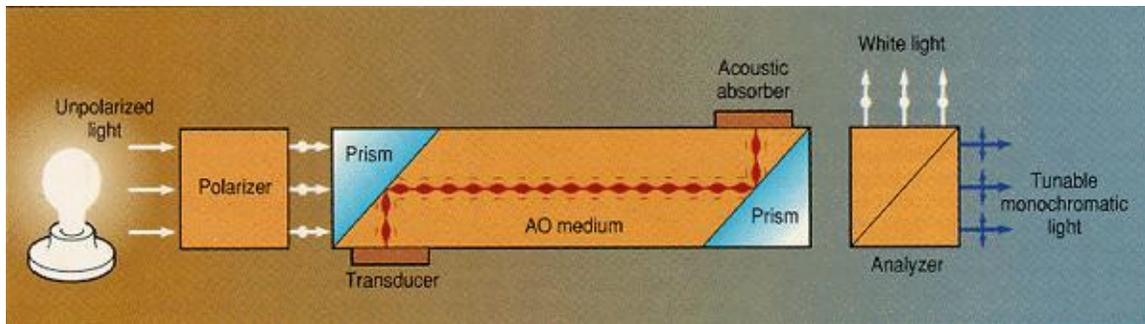
**Figure 1.** In a collinear AOTF, light waves and acoustic waves interact to produce photons at the sum and difference energies.
