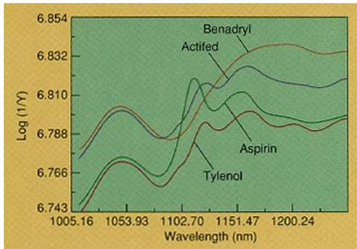
**Figure 4.** NIR reflectance spectra of common nonprescription tablets sealed in a glass bottle, recorded with a Brimrose Free Space spectrometer, reveals differences in tablet composition.
