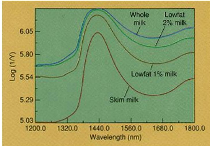
**Figure 3.** NIR reflectance spectra of various milks, recorded with a Brimrose Free Space spectrometer, indicate fat levels during processing.
