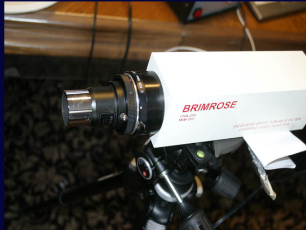
Imaging Spectrometer attached to a spotting scope:
