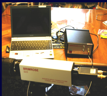
550 nm to 1000 nm Acousto-Optical Tunable Filter set up to take hyperspectral images of oranges
