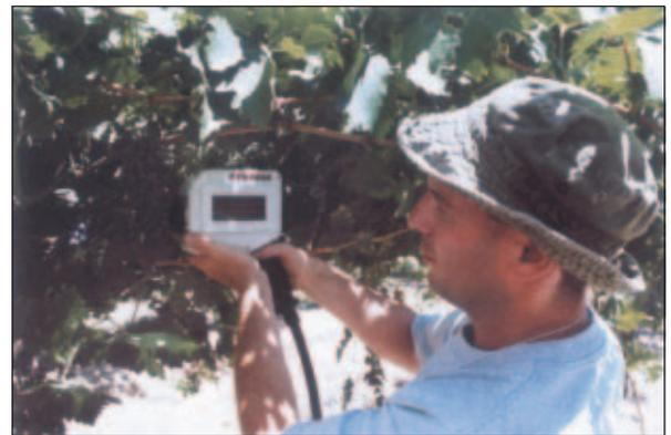
VERC research assistant **Oren Kaye** demonstrates a Brimrose NIR spectroscopy hand-held unit that can take readings for Brix, pH, TA, etc. from any grape in the vineyard without removing it from the vine.
