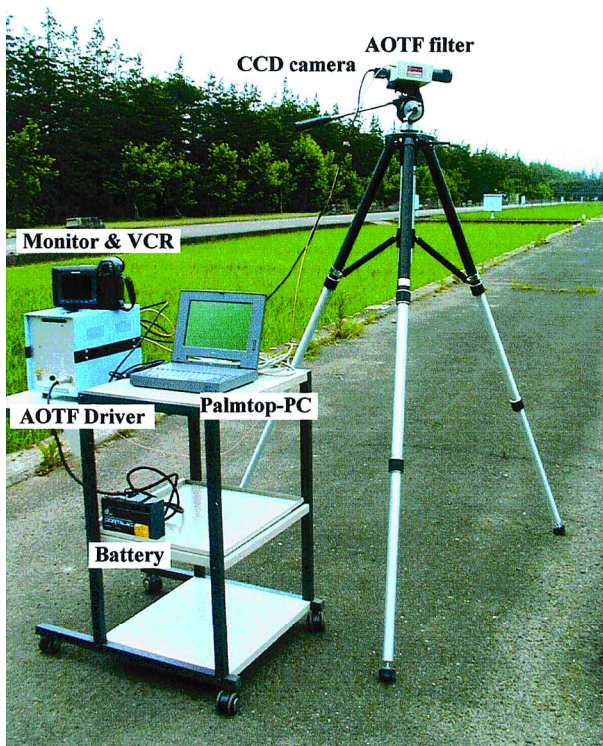
Figure 1. The AOTF-based spectral imaging system for field use.
